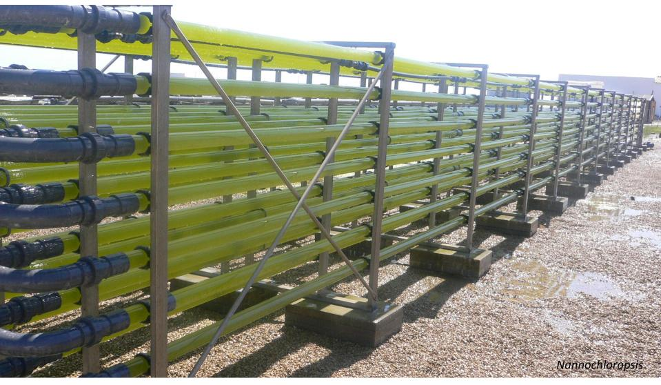
Tubular photobioreactors designed and built by Necton are in continuous operation everyday, every year since **2005** to present. Several microalgae are grown in this PBR and harvested with a centrifugue.
