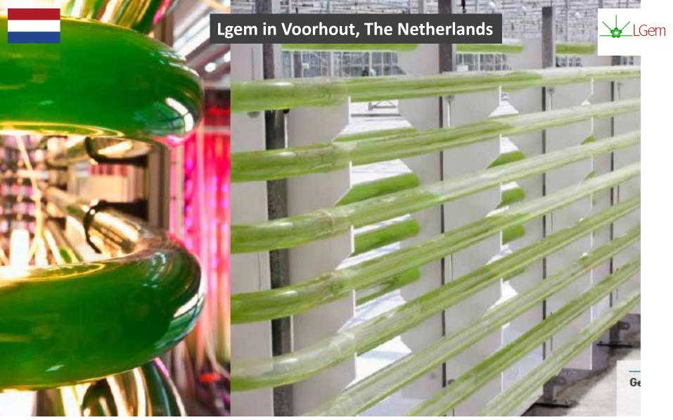
LGem is the first Dutch company to use closed photobioreactors to produce microalgae on a commercial scale. Since 2007 freeze-dried algae powder has been produced and sold all over the world as a food supplement. In 2009, GF Piping Systems joined the development team, introducing new components. As a result of this fruitful collaboration, the tubular PBR has evolved into a cleverly designed system, with low operating costs.
